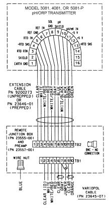
FIGURE 2-27. Wiring Model 396VP and 398VP to Model 3081, 4081, and 5081 through a Remote Junction Box
